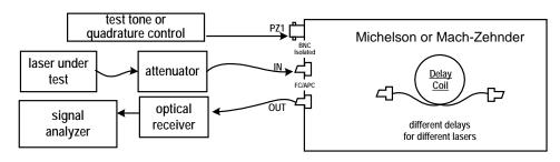
Laser under test is input to interferometer, which is set to the appropriate optical path mismatch by selection of the delay line which may be user installed or changed. Voltage control is applied to the PZ1 fiber stretcher input to maintain quadrature bias. Output optical signal is applied to an optical receiver. Receiver output to a signal analyzer or digitizer / recorder.
