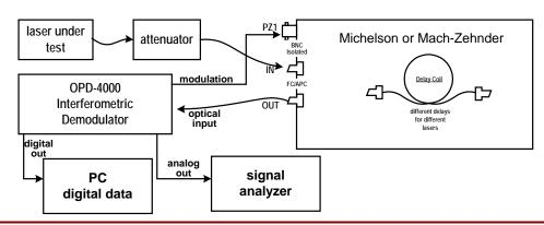
Laser under test is input to interferometer, which is set to the appropriate optical path mismatch by selection of the delay line which may be user installed or changed. OPD-4000 modulation output is applied to the PZ1 fiber stretcher input. OPD-4000 phase measurement output is selected as either digital or analog. Digital data is post processed. Analog data is available made to signal analyzer.
